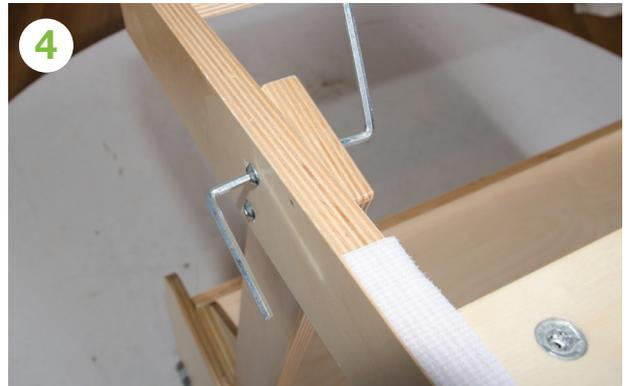
Tighten long bolts into insert nuts with 2x Allan keys provided. Repeat steps 1 and 2 on opposite end.
